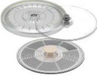
The image shows a rotor assembly for a hematology analyzer. It consists of a circular base with a central hub and a transparent cover with a scale around the perimeter. A thin tube is connected to the center. | Ротор AC24 на 24 гематокритных капилляра, с крышкой и шкалой |
